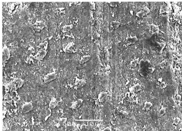
Fig. 3. SEM observation of fractured surface of Group PV with fatigue loading (original magnification \times 2000 ).
